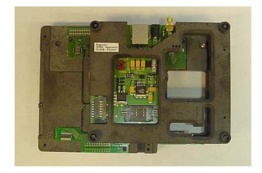
*Note: The nominal supply voltage for MJ-25 is +6.0 V.*  The supply voltage must not exceed +12.0 V (min. 5.0 V). Supply the power to jig only when the jumper is open = regulated.
