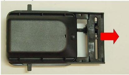
2 Insert the adapter to the phone from battery connector side.
